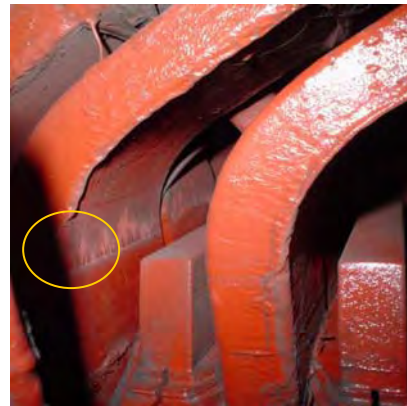
Figure 1 – Signs of discharges on a winding after just four years of service
